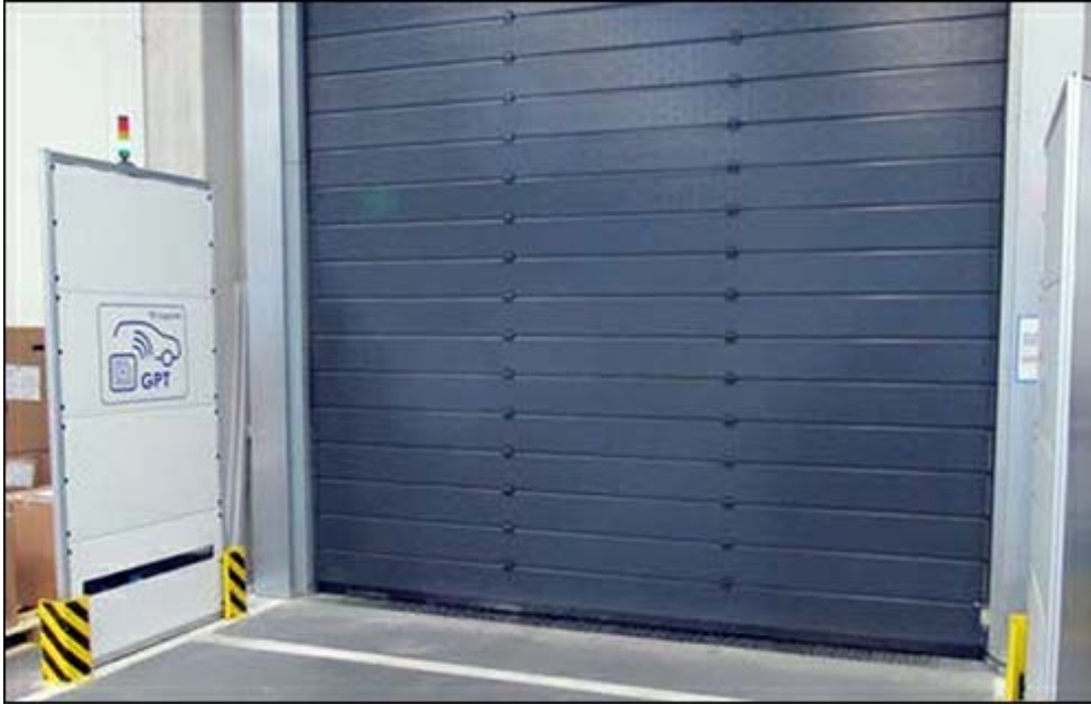
Figure 1: RFID in Incoming Goods —The RFID-tagged prototype parts are automatically recorded in the incoming goods department.
