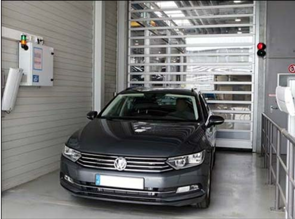
Figure 2: RFID in Vehicle Testing —Volkswagen AG's technical development department reads test vehicles using RFID gates. This involves a combination of side and ground antennas that enable an instant 360-degree inspection. The data from the RFID-tagged prototype parts is communicated to IT systems that support the process. This results in automated construction documentation, which does away with the need for many previous manual operations.
