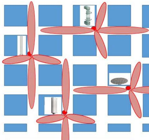
Figure 2 Network Layout Using Buildings to Isolate Small Cells to Reduce Interference and Optimize Performance. Fitting Antenna to the location allows better coverage and less Antennas.
