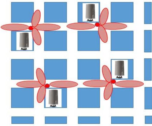
Figure 1 Network Layout Needing Adjustable Electrical DownTilt to Reduce Interference and Optimize Performance. AEDT reduces Small Cell coverage requiring more Antennas.
