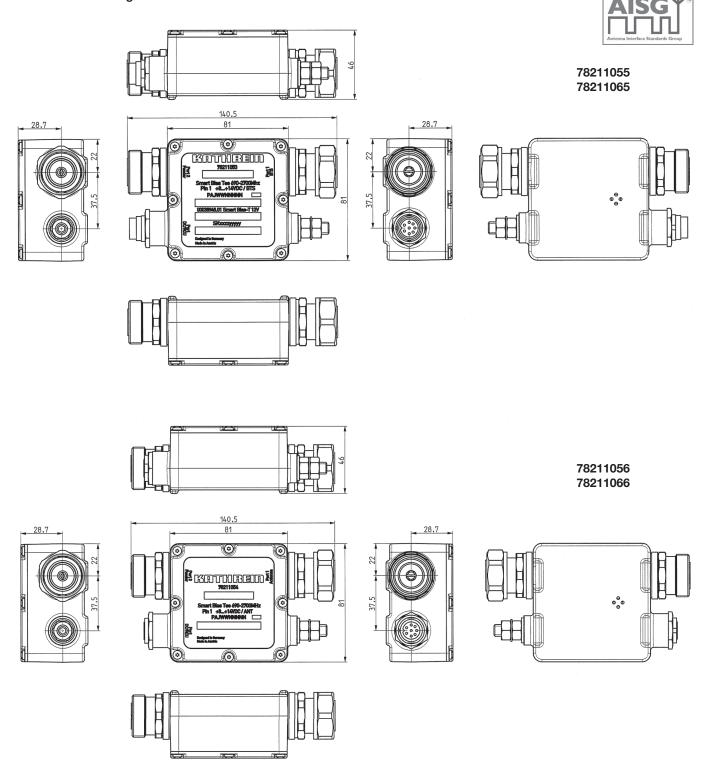
The Smart Bias Tees are designed to operate under the environmental conditions as described in ETS 300 019-1-4 class 4.1 E and have passed environmental tests as recommended in ETS 300 019-2-4.
