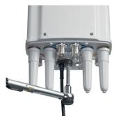
For the feederline installation carefully put the connector in place and hand-screw the nut.
