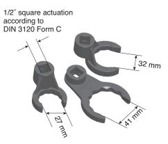
These tools are suitable for 7-16 connectors with a wrench size of 27 or 32 mm, and the RCU attachment nut with a wrench size of 41 mm.
